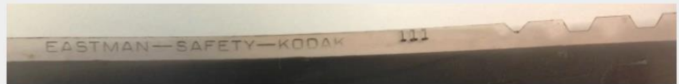
An example of edge printing and notch codes for an acetate negative. Photo credit: Amanda Oliver
