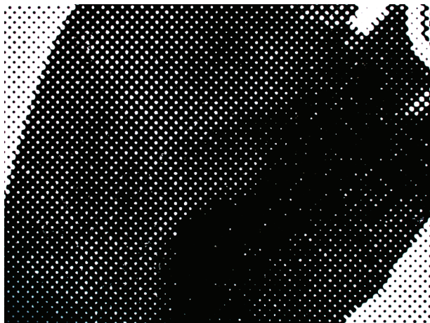
Figure 8g Letterpress halftone print at 50 lpi created using an Ives/Levy halftone screen (6.3× magnification in the Dmax area).
