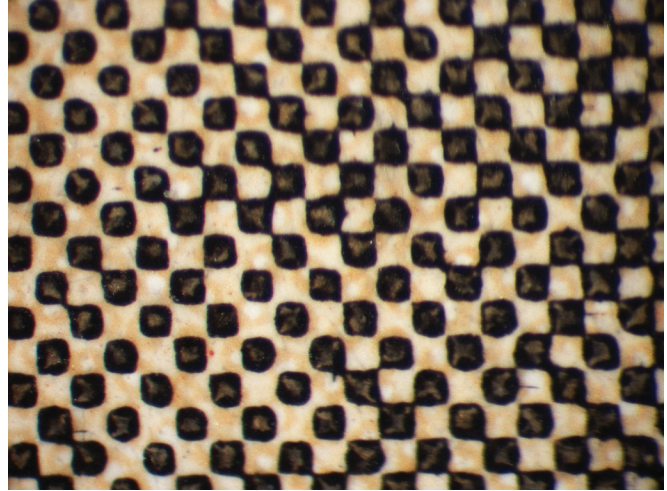
Figure 12b Detail of the lighter area of the print in fig. 12a, showing the dot pattern using a light color ink overprinted with a black ink (80x magnification).
