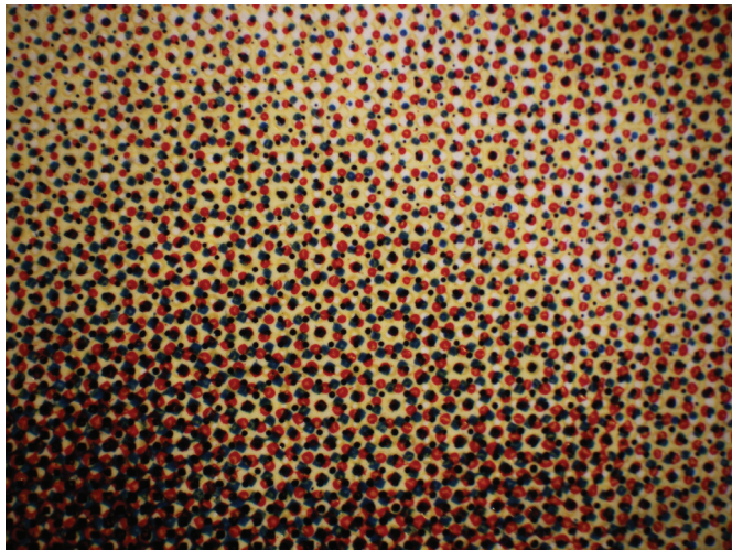
Figure 21b Microscopic detail of fig. 20, recorded at 25× magnification, showing superposition of all four color print layers.
