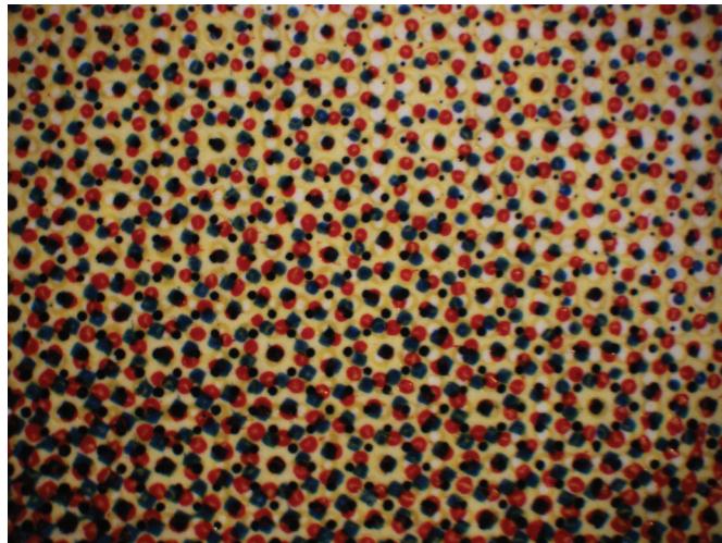
Figure 21c Microscopic detail of fig. 20, recorded at 40× magnification, showing superposition of all four color print layers.
