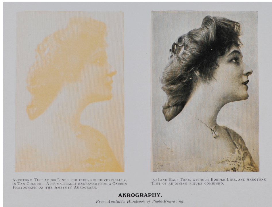
Figure 31 Photo-mechanical print, 1908, made using the so-called Akrography process.
