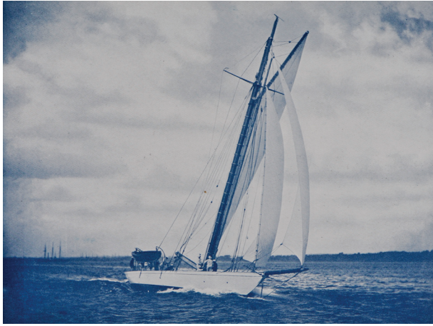
Figure 10c Halftone print created using a standard Ives/Levy halftone screen at 150 lpi.
