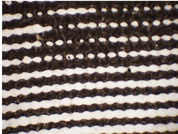
Figure 30a Microscopic detail of the wavy-line screen pattern at 6.3× magnification.
