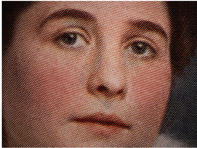
Figure 16a Microscopic detail of fig. 14, recorded at 10× magnification, showing superposition of all three color print layers.
