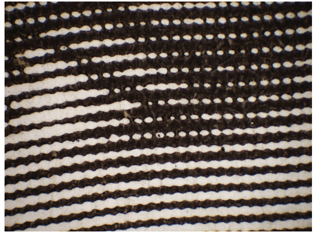
Figure 30b Microscopic detail of the wavy-line screen pattern at 25× magnification.
