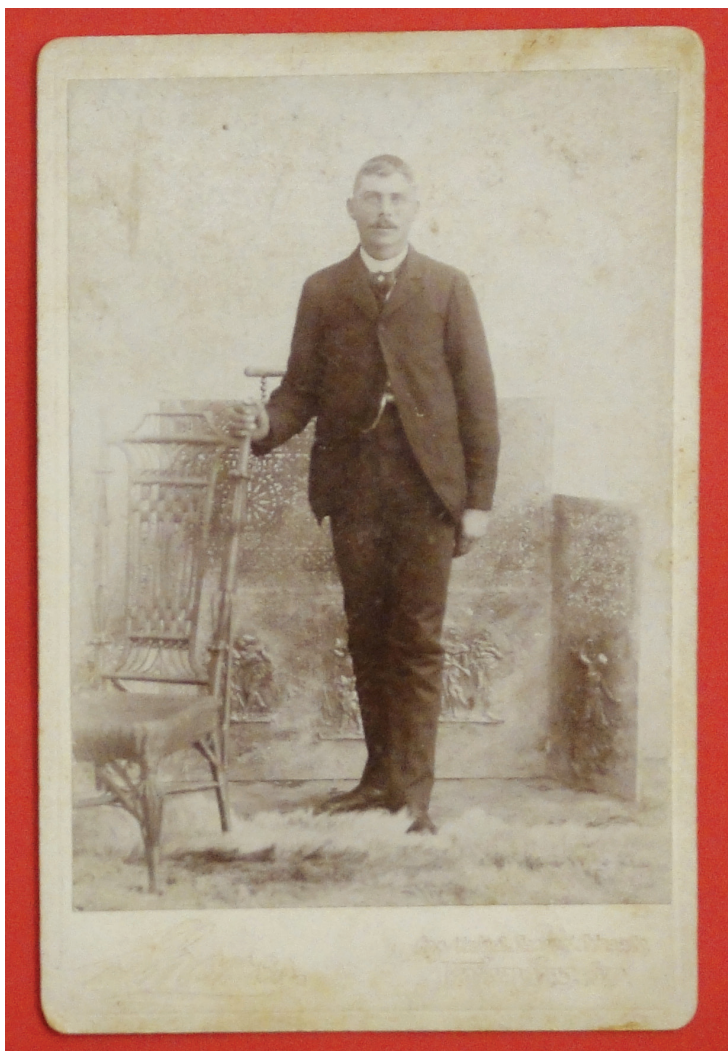
Figure 18 CC-mounted glossy collodion photograph treated with a beeswax-based varnish to produce a matte surface.
