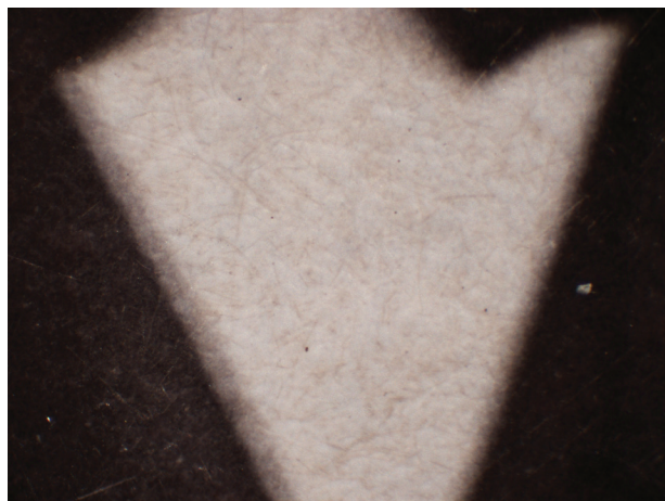
Figure 10a Detail of the Dmin area of the photograph in fig. 6 at 40x magnification, showing fibers in the paper substrate.
